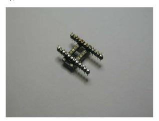
Now place the pcb on top of the headers, so that the pins are in the P1 holes, as shown below, and solder them. Just solder two pins first, then check to make sure that the pcb is sitting properly before soldering the rest of them.
