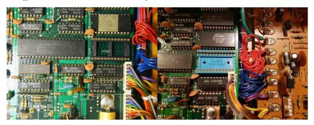
The adapter board and headers have been designed to work with either type. The one on the left has machined contacts, while the Yamaichi one on the right has stamped contacts.
