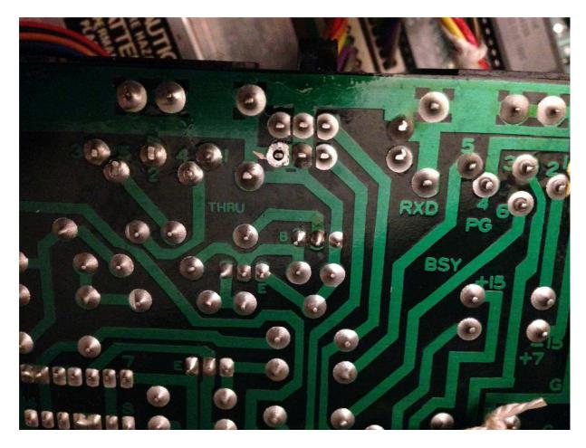
One possible problem with this approach is that the switch pin may move a little as the switch setting is changed, so even though it appears to be isolated, it could possibly re-connect by accident, causing mysterious problems.
