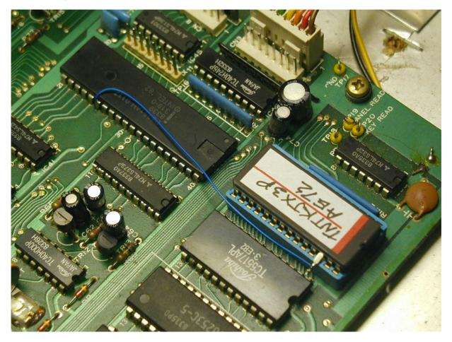
Roland designed the JX-3P to use the PG-200 for patch editing. As a result, memory is protected with the Protect switch in the MIDI position, as well as in the Protect position. The new firmware needs to be able to write to this memory with the switch in the MIDI position. There are three ways this can be accomplished:
