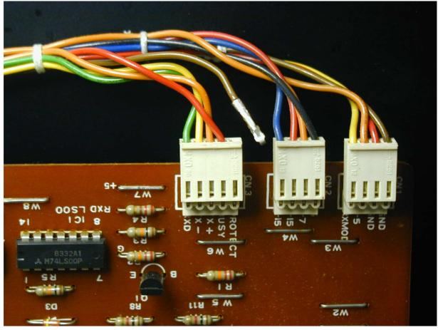
3) The above two methods leave memory unprotected in all three switch positions. It is also possible to modify the jacks board so that MIDI will be unprotected, but in the Protect position memory will be protected. To accomplish this, one pin of the Protect switch must be isolated from the circuit board trace. Here is a photo showing how this looks on the later version of the jacks pcb:
