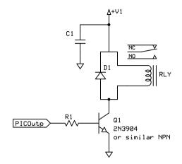
R1 should turn on transistor hard enough to keep "on" state power dissipation low.
