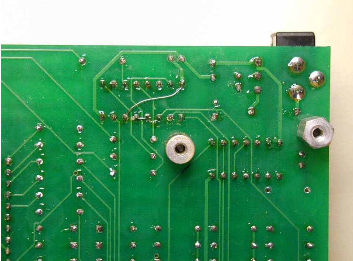
There is one jumper from U5 pin 6 to U5 pin 16, and also U5 pins 4 and 5 are shorted together. Please install these jumpers with the socket for U5 empty. **Note: These mods are not required and should not be performed on the V1.1 pc boards.**
